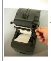
Close the lid, making sure the lid locks into place. The printer automatically feeds and cuts the paper, after the printer test. If the paper comes out blank, it has been loaded in the printer backwards.
